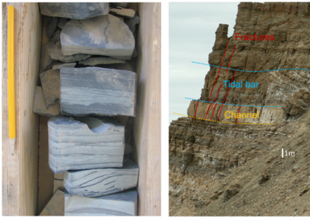
Fig. 5. Geological studies in storage-site characterization: (left) example core samples from a tidal delta lithofacies from the Carboniferous storage unit at Krechba, Algeria; and (right) outcrop analogue of tidal deltaic sedimentary architecture from the Middle Jurassic Neill Klinger Formation, Greenland. (Photographs courtesy of Phil Ringrose.)
